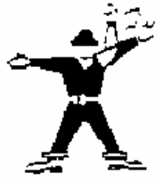
MOVE LEFT Right arm horizontal Left arm sweeps upward to position over head
