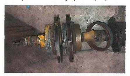
removing the pump housing it was discovered that the pump impellor was damaged and destroyed on the 31 year old truck. Engine 1932 is a 1986 Pierce Dash truck and is our second out truck here at Station
